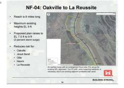
NF-04 is Oakville to La Reussite and this reach is eight miles long. The maximum existing height is at elevation 9. Again, we will be raising these to provide a 2% level of risk reduction in this area and the elevations will range from 7.5 to 9. As you can see these are the communities included in the reach that will have a reduced risk.
