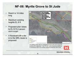
NF-06 is Myrtle Grove to St. Jude. This reach is 14 miles long and the maximum existing height here is 6 feet and the propose plan will raise it to elevation 12. This red box right here shows where we currently anticipate based on available funding to tie into the Mississippi River Levee.
