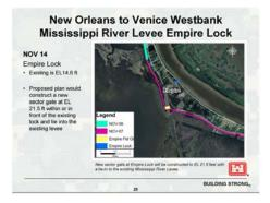
NOV 14 is the Empire Lock. This plan is to construct a sector gate at elevation 21.5 and the current plan would be to place a sector gate within the existing structure and tie into the levees on either side. The existing elevation right here is 14.6 so it will gain about seven feet of protection right there.
